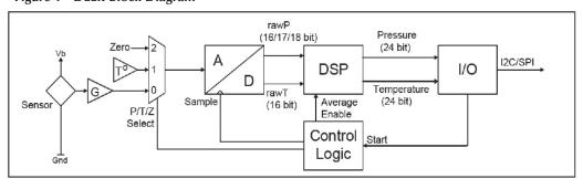
The ADC performs conversions on the raw sensor signal (P), the temperature reference (T) and a zero reference (Z) during the ADC measurement cycle.
